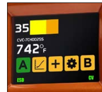
Tip temperature displayed on large color screen.
